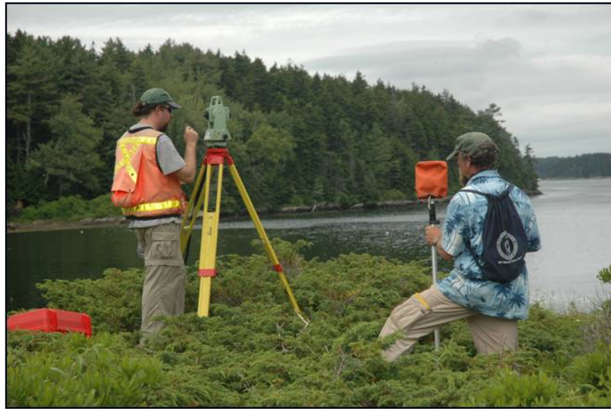
One of our 2007 field school students Seth, was an experienced land surveyor. Here he is at left using an electronic surveying instrument (“total station”). I am at right preparing to deploy the reflector unit. Bear Island is across from us.
